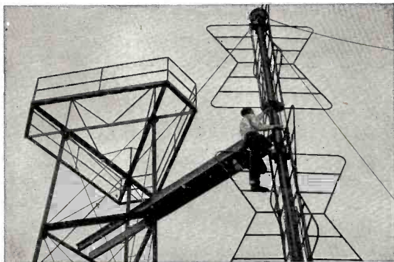
Performance-engineered antenna is run through rigorous G-E checks at factory. To simulate operating conditions, special tower at Syracuse was rigged to run exhaustive in-service tests before antenna was flown to customer.
